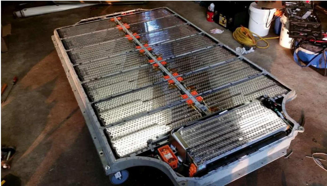
Bild 1. Akkumulator eines Tesla Model S. https://www.forbes.com/sites/arielcohen/2020/12/30/teslas-new-lithium-ion-patent-brings-company-closer-to-promised-1-million-mile-battery/#2b03662f33e3
